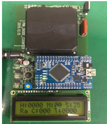
Figure 9. Radon counter implemented using an arduino MCU module
